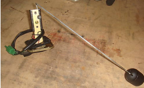
Fuel sensor with float
