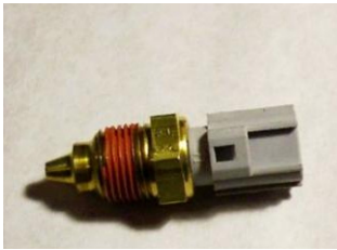
Coolant temperature sensor - single resistor type
