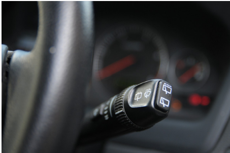
Indicator stalk houses several types of switch
