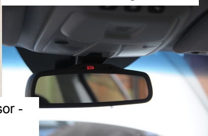
Mirror with internal light sensor
