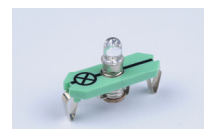
LED bulb with internal current limiting resistor
