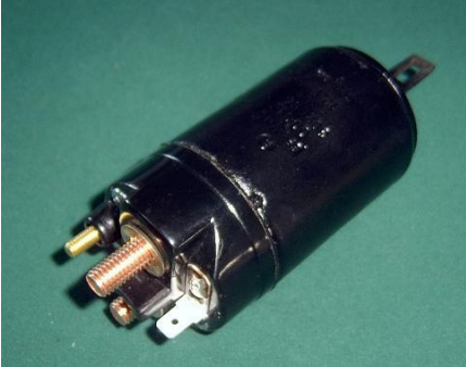
Typical starter motor relay - often called a 'solenoid'
