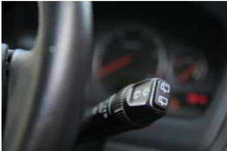
Indicator stalk houses several types of switch
