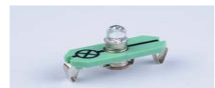
LED bulb with internal current limiting resistor
