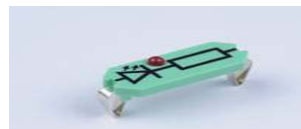
LED with current limiting resistor
