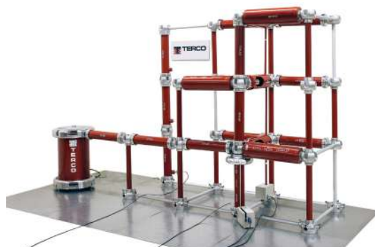
3-stage DC Voltage Test Set-up
