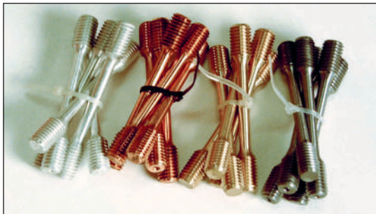
Sets of Tensile Test Rods
