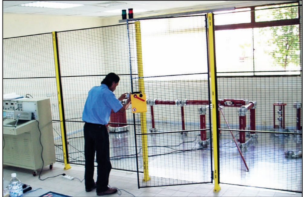
Power Supply for HV9000 is 220/230V, 50/60Hz single phase. Fuse 25A D characteristic.
